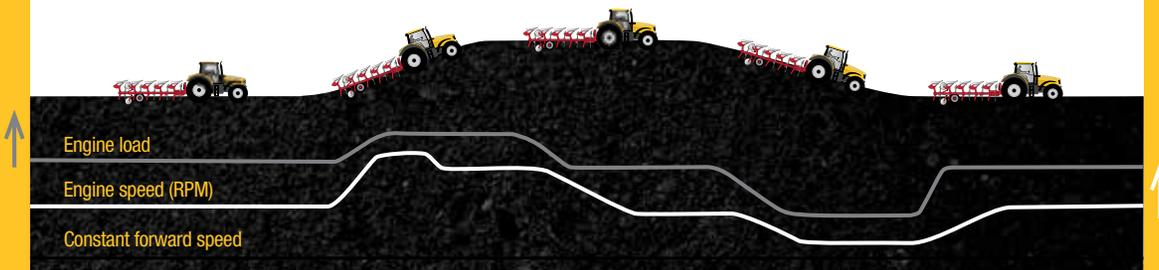
As the load (grey line) varies according to conditions, the TMS will automatically adjust the engine speed (white line) to maintain the forward speed while minimizing fuel consumption and noise levels.
